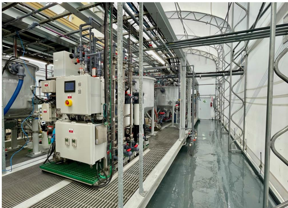
Figure 2. SiFT pilot plant installed and integrated with the existing DLE plant inside the weatherproof structure in El Dorado, Arkansas. (Photo from the Standard Lithium Ltd. news release dated on September 1, 2021)
